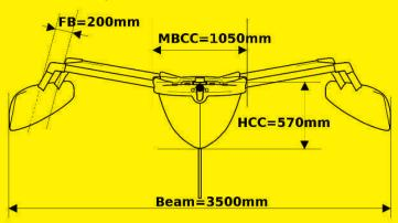
Diagram 3: Dimension of Hulls - Front View
