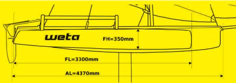
Diagram 2: Dimensions of Hulls - Side View
